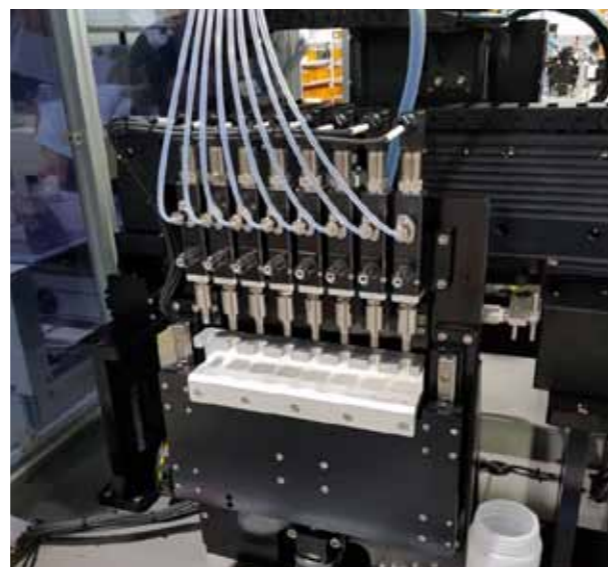
<8-ARRAY PLUNGER PUMP SYSTEM>
