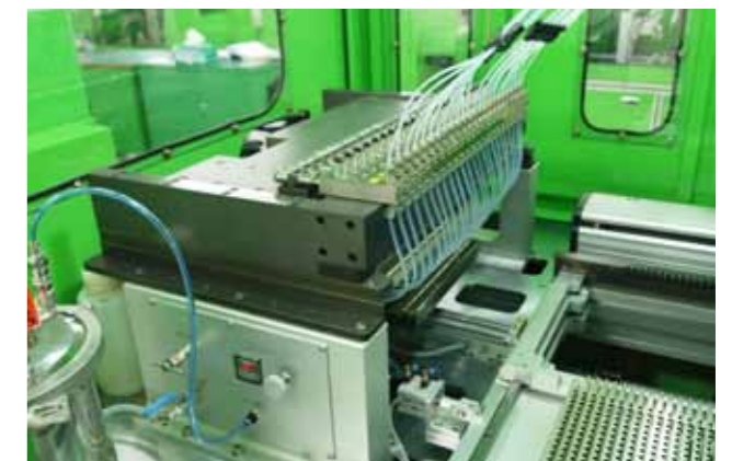
<24-ARRAY PLUNGER PUMP SYSTEM>
